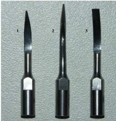
Fig. 4: Illustration of the tip types. Tip type 2 was selected to perform the cavitometer validation
